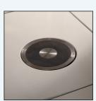
**Moisture control** Electrodes measure humidity in the concrete and automatically regulate addition of water via SKAKOMAT 600.
