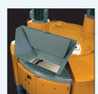
Water proportioning Water proportioning device enables the addition of water during production. Different models available for different types of concrete.
