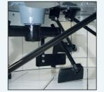
Unique two-level shovel technology ensures better controlled high intensive mixing. Bolts are countersunk so concrete will not stick and old concrete will not get
